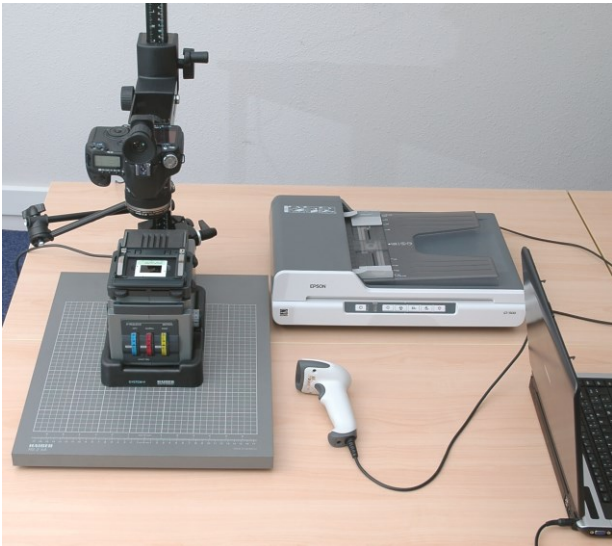
Digitization System showing copy stand, slide holder, barcode reader, scanner and computer system.
