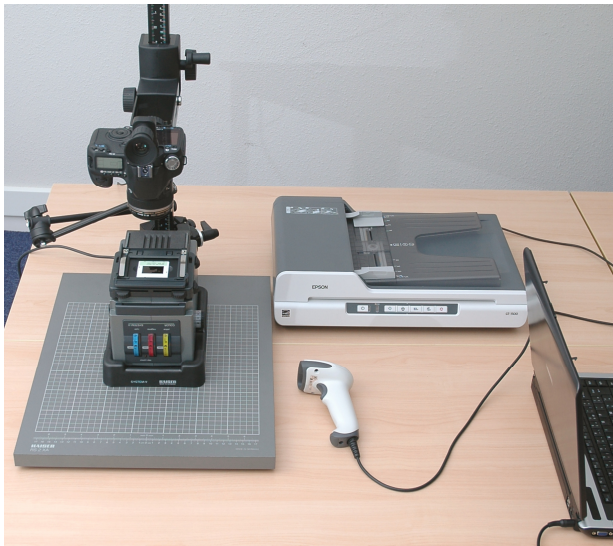
Digitization System showing light stand, slide holder, display and computer system.
