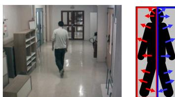
Our method is based on pedestrians appearance in images. The gradient orientations are used as shape features. In order to speed up the detection our approach is based on a cascade of classifiers:
