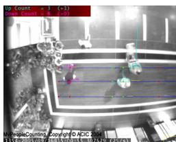
Detects moving people on a set of detection lines. Once it is possible to group a detection on each line, the algorithm considers that a person can be counted.
